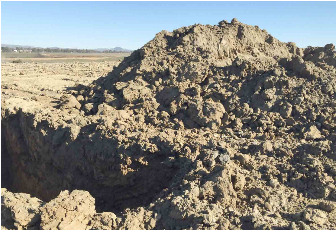
Photo No. 10 Test Pit TP2 in Borrow Area #2 (Silt)
